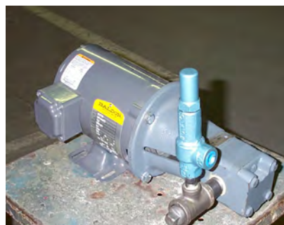
Figure B-13 Oil Pump and Regulator
