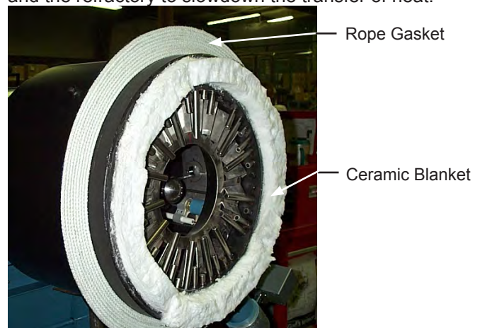
Figure B-11 Gas Manifold
