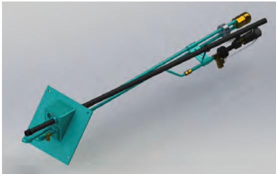
Figure B-8 Burner Drawer Assembly
