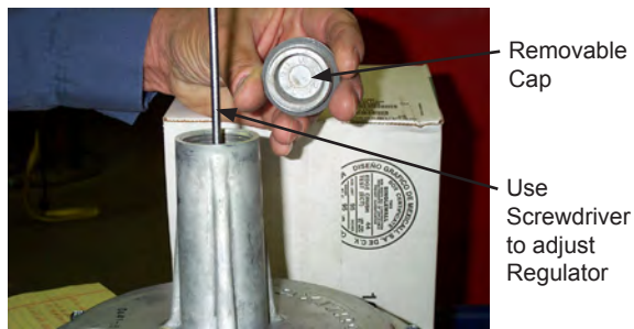
Figure E-7 Main Gas Pressure Regulator Adjustment
